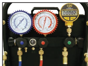
Hard mounted manifolds
