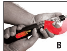
B Rotate handle to select bit
